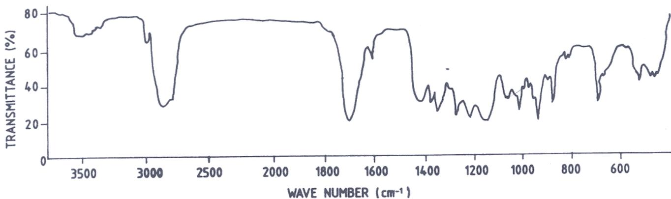
Figure 1. IR spectrum of HTBCP.
