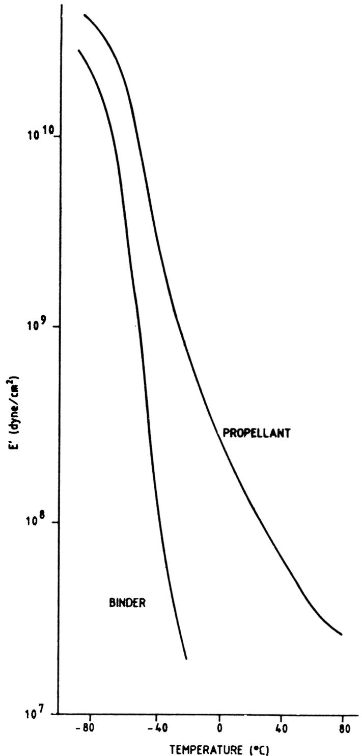
Figure 3. Comparison of storage modulus of PBAN propellant and binder at different temperatures at 35 Hz.
