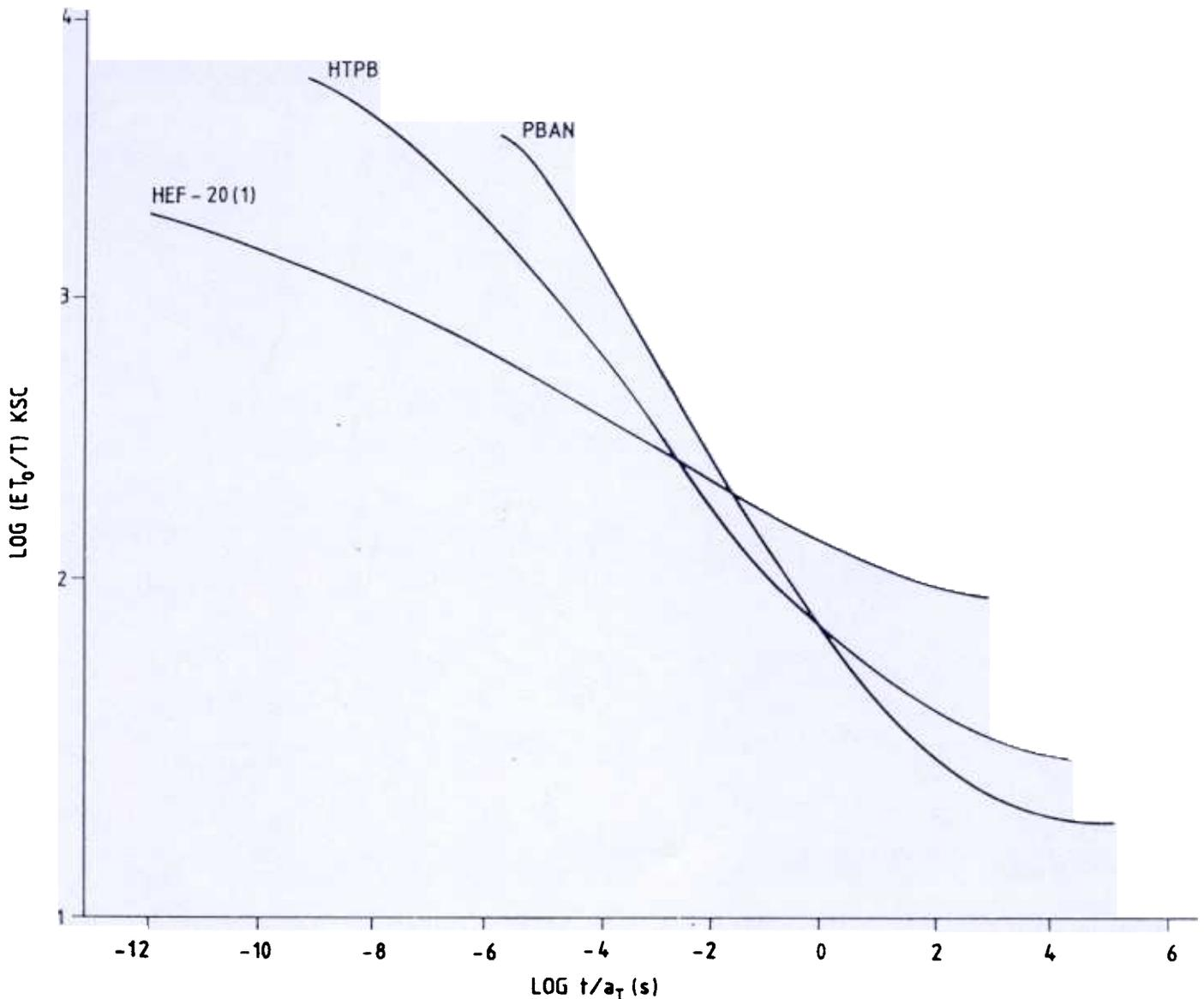
Figure 8. Comparison of master curves for three propellants.
