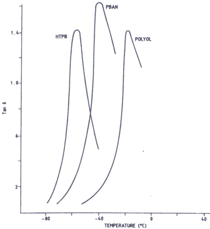
Figure 2. Dependence of loss tangent on temperature at 35 Hz for various polymeric binders.
