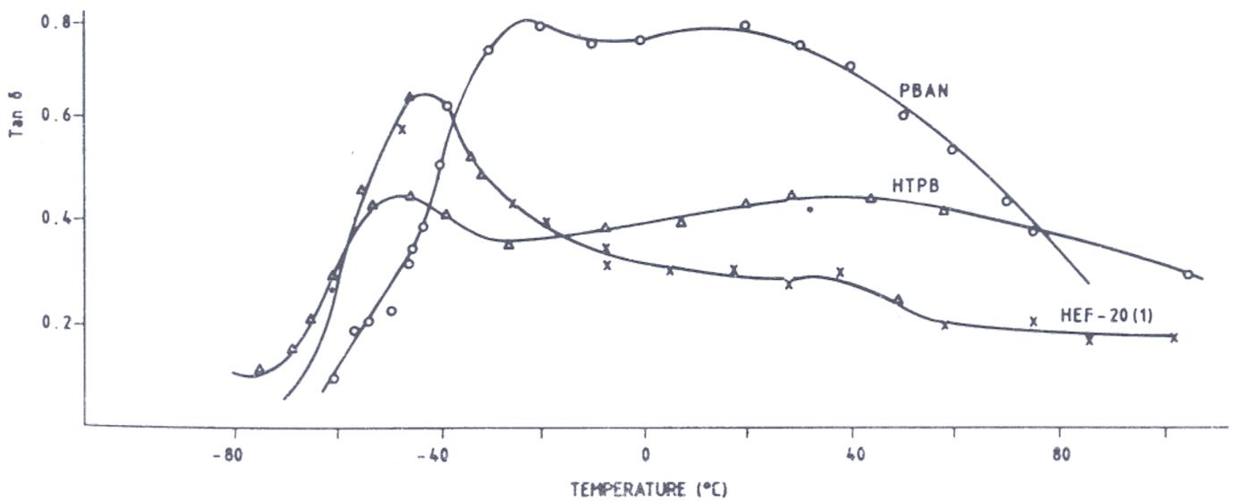
Figure 6. Comparison of loss tangent data of different propellants at different temperatures at 35 Hz.
