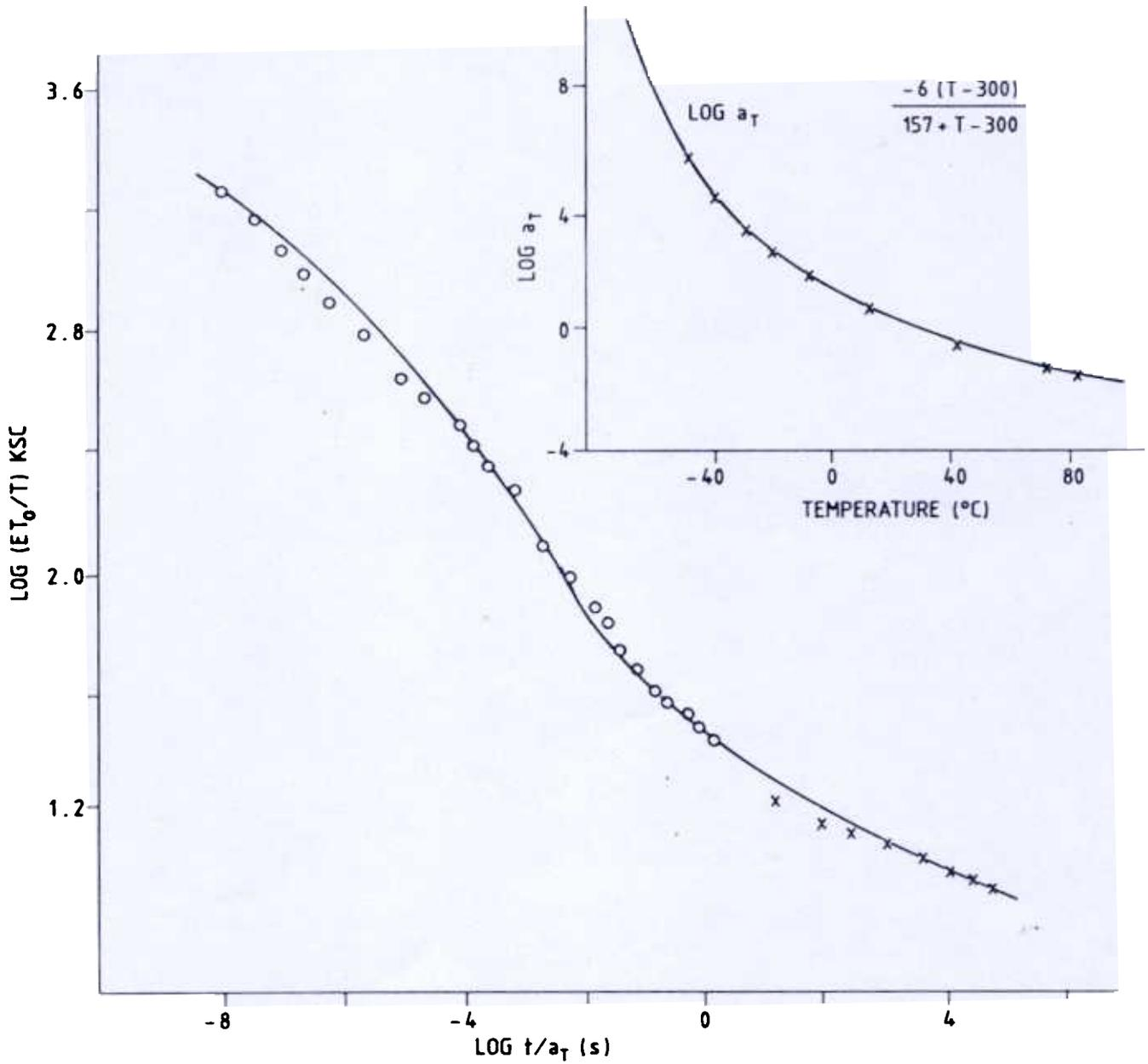
Master curve for HTPB propellant using 300 K as reference temperature. Inset figure shows dependence of shift factor ( $a_T$ ) on temperature
