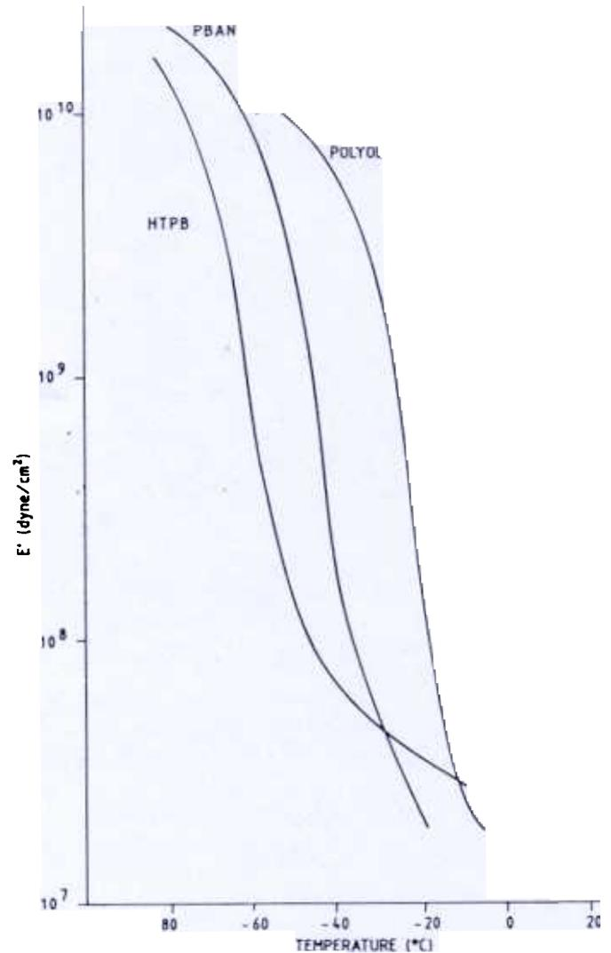
Figure 1. Dependence of storage modulus ( $E'$ ) on temperature at 35 Hz for different polymeric binders.
