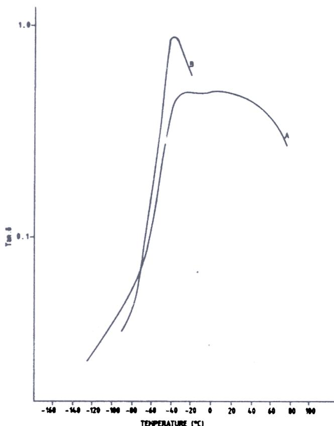
Figure 4. Comparison of loss tangent of PBAN propellant (curve A) and binder (curve B) at different temperatures at 35 Hz.
