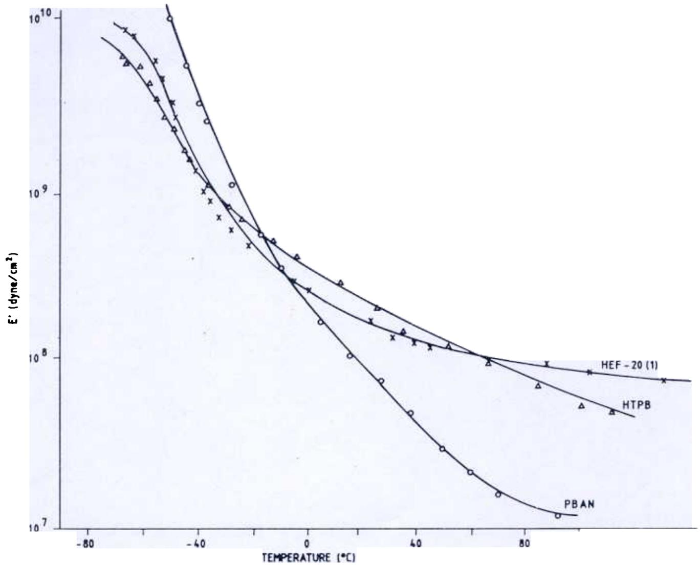
Figure 5. Dependence of storage modulus ( $E'$ ) on temperature for different propellants at 35 Hz.
