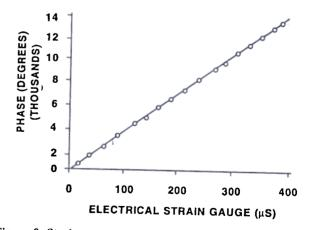
Figure 9. Strain response of a MFO strain sensor embedded within a carbon/PEEK thermoplastic cantilever beam.
