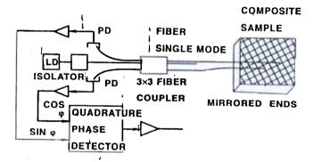
Figure 2. Schematic diagram of Michelson fiber-optic sensor based on passive quadrature detection by means of a  $3 \times 3$  coupler.
