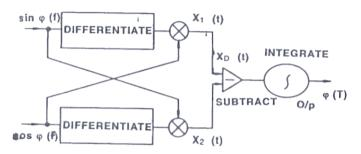
Figure 3. Differentiation and cross-multiplication demodulation scheme.
