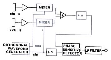
Figure 4. Orthogonal carrier wave demodulation technique.
