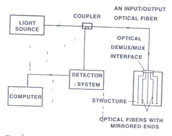
Figure 8. Generic Fiber-optic smart structure involving a light source, coupler, an input/output optical fiber (or bundle), optical fiber sensor array, the detector system and the interrogation system with computer.
