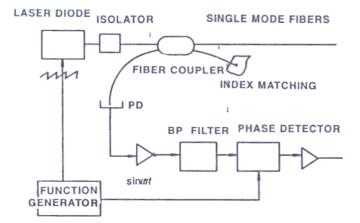
Figure 6. The signal recovery system for a FPFO sensor based on linear wavelength ramping of the laser diode.
