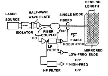
Figure 5. Set-up for piezoelectric active phase-demodulated MFO sensor employed for acoustic emission detection.
