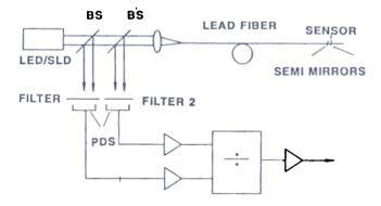
Figure 7. Spectral ratiometric demodulation for a FPFO sensor with a large FSR.
