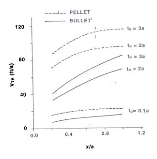
Figure 4. Threshold velocities for spherical and paraboloidal projectiles of same mass for different values of skin thickness.
