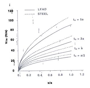
Figure 2. Threshold velocity V<sub>th</sub> (ft/s) for the age group 30-50 years for different values of skin thickness.
