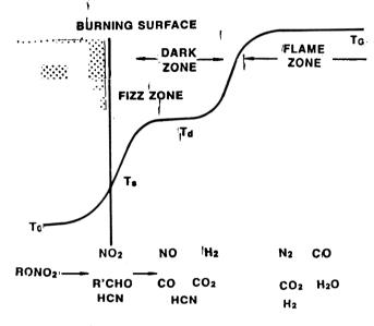
Figure 2. Schematic diagram of the flame structure (combustion wave) nitramine double base propellant.
