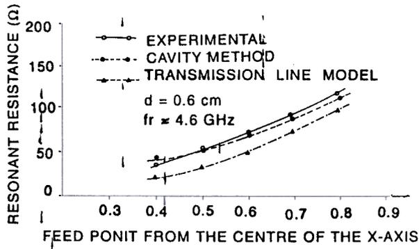
Figure 3. Variation of resonance resistance with feed location along x-direction at  $TM_{11}$  mode.
