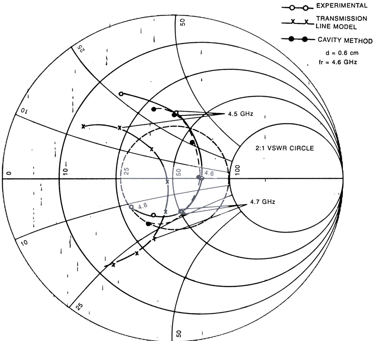
Figure 5. Impedance pattern at  $TM_{11}$  mode (feed position  $d = 0.6$  cm, where maximum band width is obtained).
