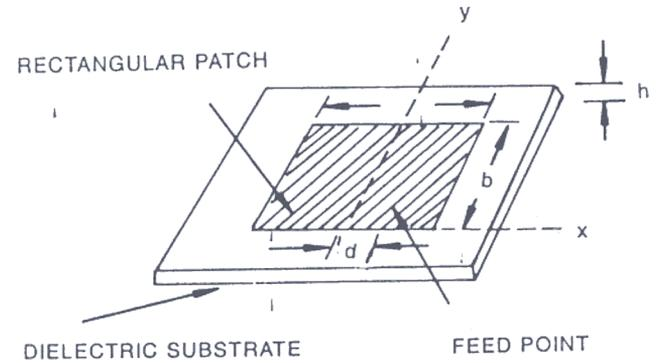
Figure 1. Rectangular microstrip antenna.
