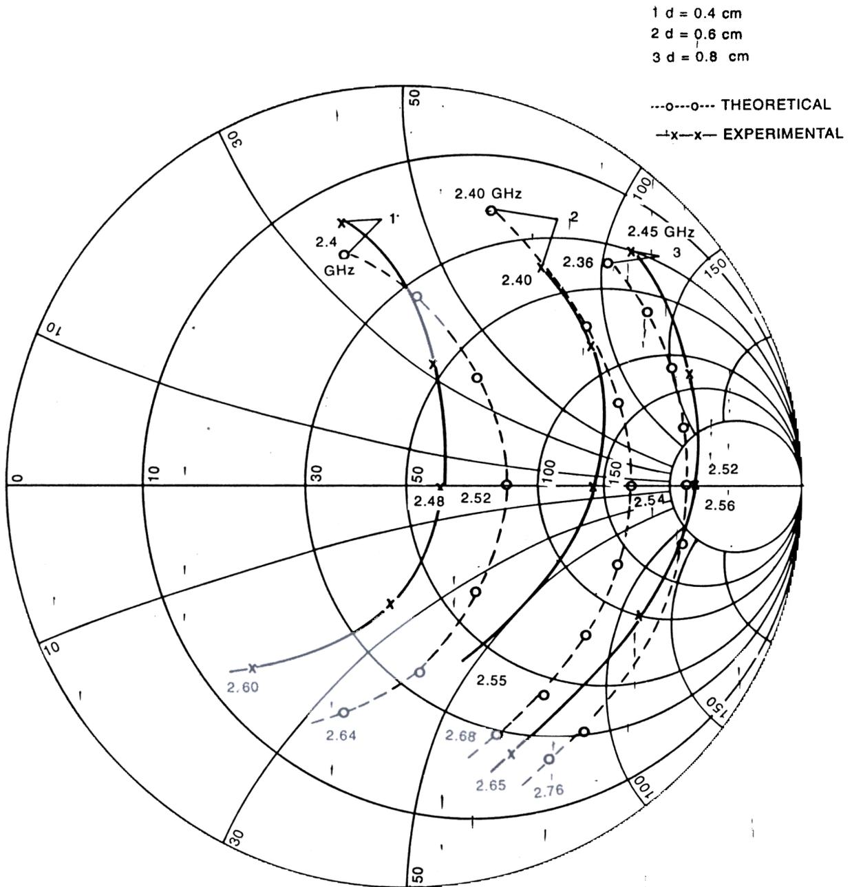
Figure 2. Variation of Input Impedance with feed location at  $TM_{10}$  mode.
