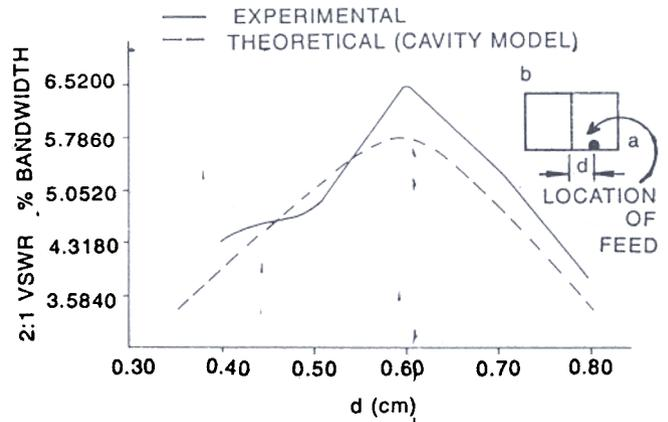
Figure 4. Variation of 2:1 VSWR impedance bandwidth with feed location at  $TM_{11}$  mode.
