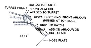
Figure 3. Upward-opening, front armour to facilitate driver's exit.
