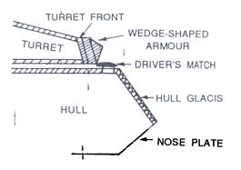
Figure 2. Wedge-shaped turret front armour.
