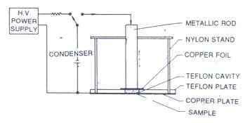
Figure 2. Schematic diagram of instrument for spark sensitivity test.
