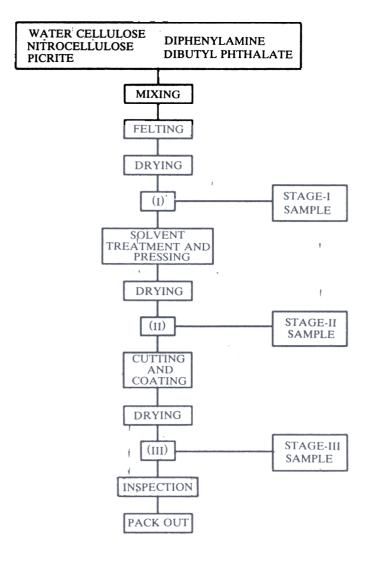
Figure 1. Combustible component manufacturing flow diagram.
