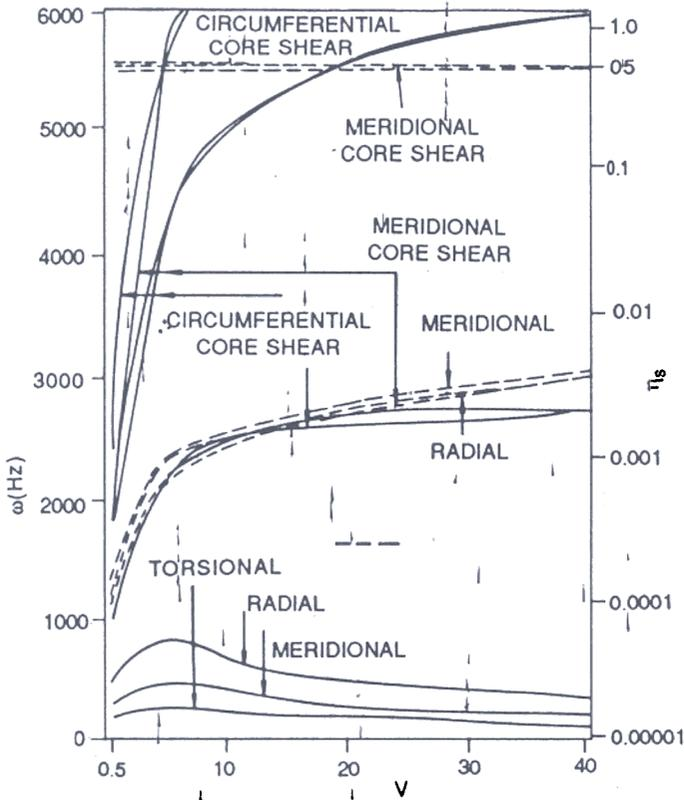
Figure 4. Variation of  $\omega$  and  $\eta_s$  with  $V$  for axisymmetric vibrations of a free-free seven-layered conical shell.
