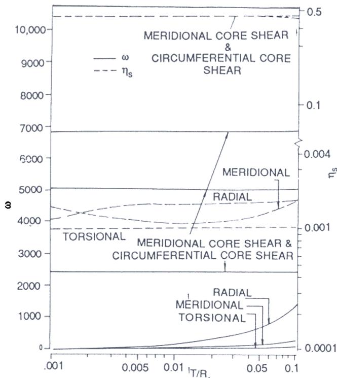
Figure 7. Variation of  $\omega$  and  $\eta_s$  with  $(T/R_1)$  for axisymmetric vibrations of a free-free seven-layered conical shell.
