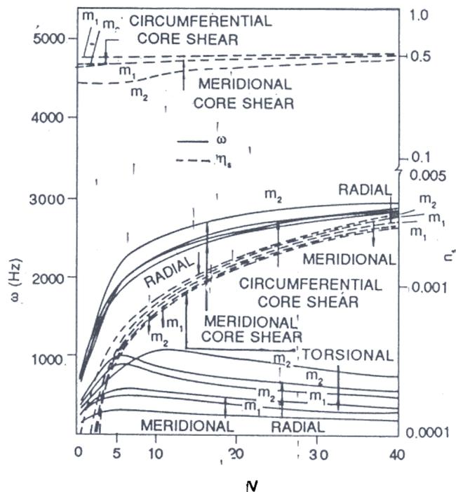
Figure 2. Variation of  $\omega$  and  $\eta_s$  with  $V$  for axisymmetric vibrations of a free-free three-layered conical shell.
