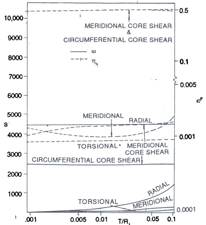
Figure 6. Variation of  $\omega$  and  $\eta_s$  with  $(T/R_1)$  for axisymmetric vibrations of a free-free five-layered conical shell.
