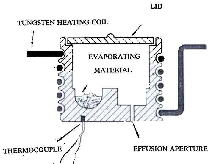
Figure 1. Vacuum evaporation crucible.
