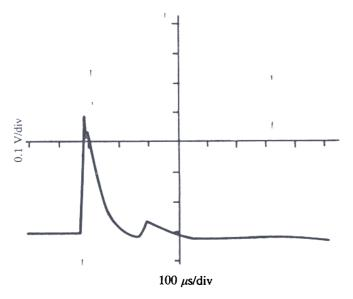
Figure 1. Pressure-time profile of shock wave in water.
