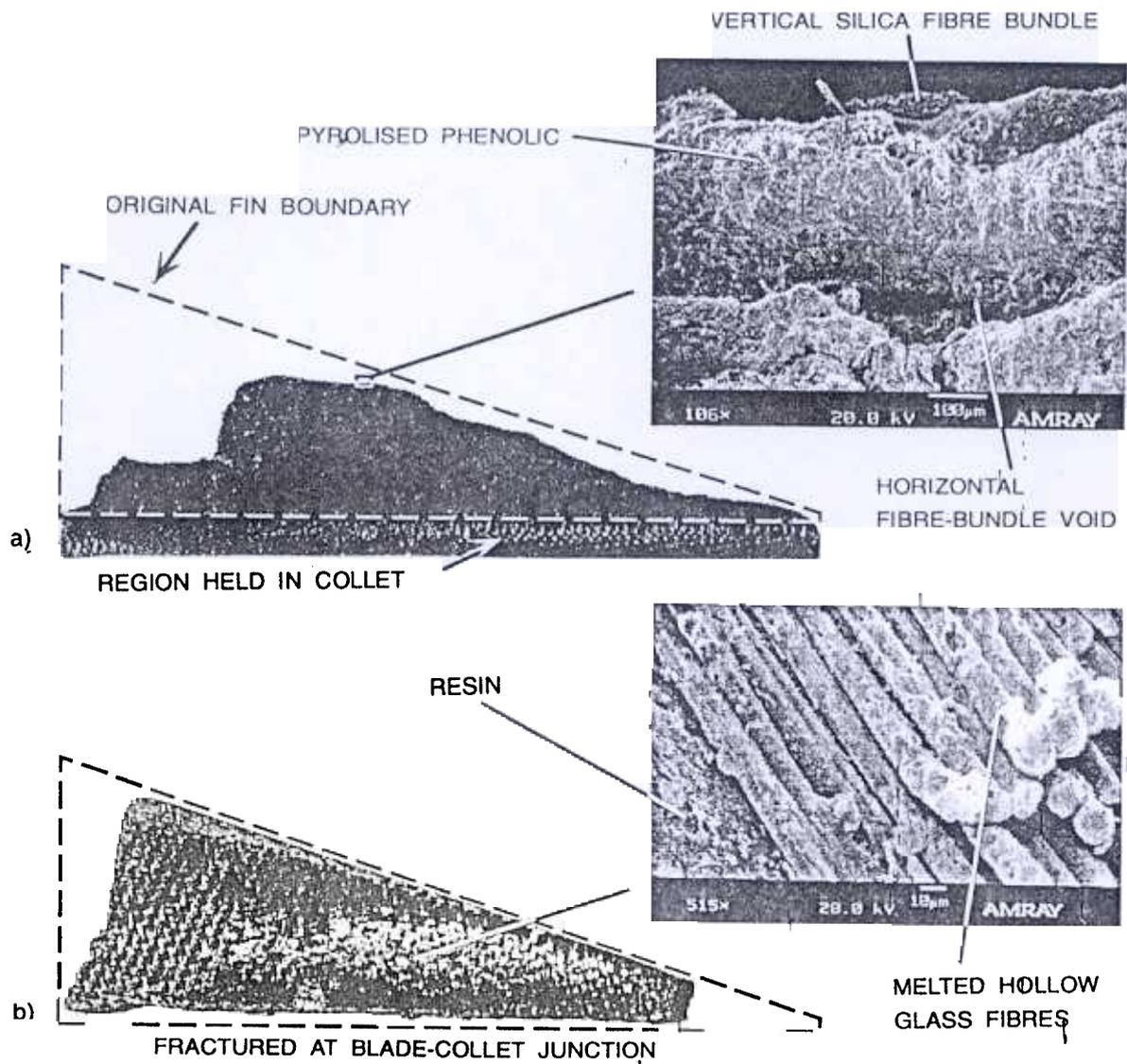
Figure 4. Static firing test results for (a) MX-2646 and (b) MXBE-55 compression-molded, fibre-filled, thermoset resins (1.52 mm blades).
