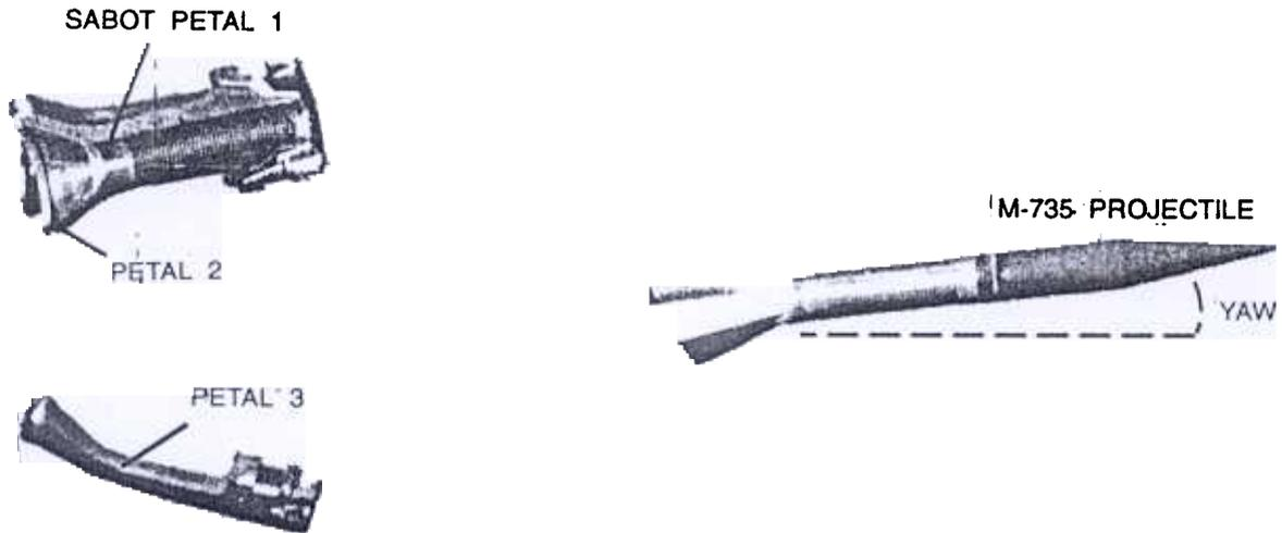
Figure 2. High speed photograph of M-735, just after sabot discard, ~ 9 m downrange from muzzle
