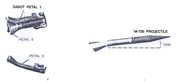
Figure 2. High speed photograph of M-735, just after sabot discard, ~ 9 m downrange from muzzle
