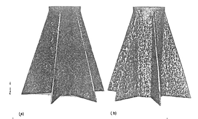
Figure 8. Static firing test result for (a) PAEK resin reinforced with 30 % E-glass fibres and (b) unfilled PAEK resin (both had 1.52 mm thick blades).
