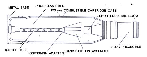
Figure Experimental setup for testing candidate fin assemblies
