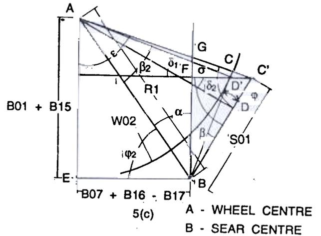
Figure 5(c). Wheel and protrusion on sear mating
