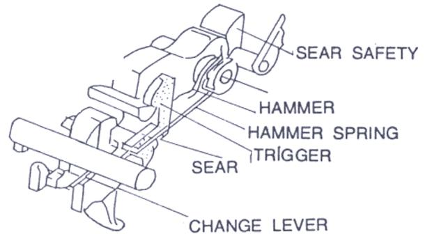
Figure 1. Firing mechanism
