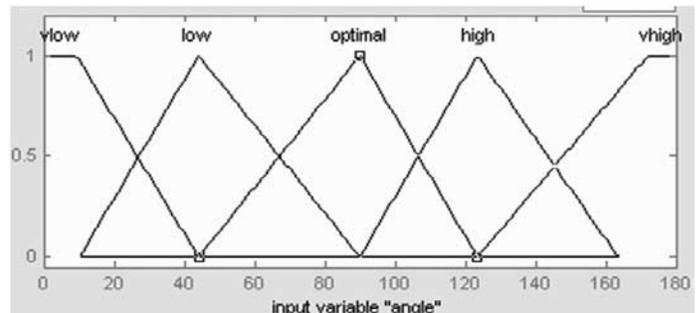
**Figure 3. Membership functions for the input angle.**
