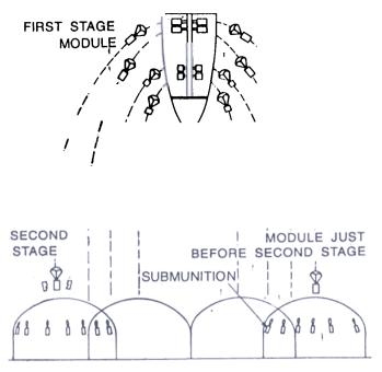
Figure 1. Two-stage ejection event
