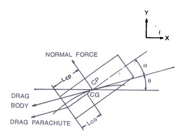
Figure 4. Force system acting on module with parachute
