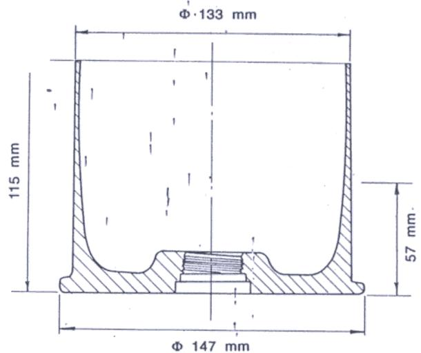
Figure 2. Brass obturator (M<sub>1</sub>)
