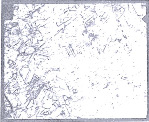
Figure 7. Micrograph taken at 25 mm distance from the lip
