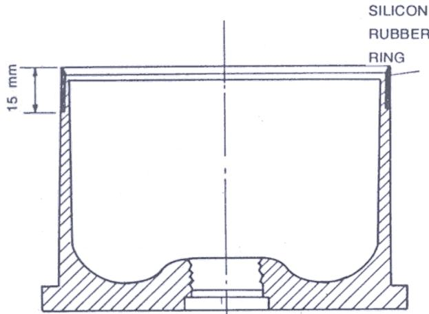
Figure 3. Brass obturator with packing material
