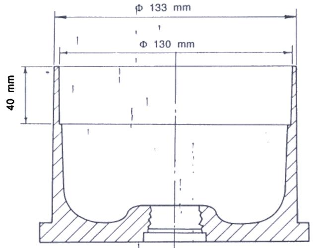
Figure 4. Annealed brass obturating cup (M2)
