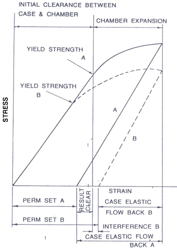
Figure 1. Case—chamber stress-strain curve
