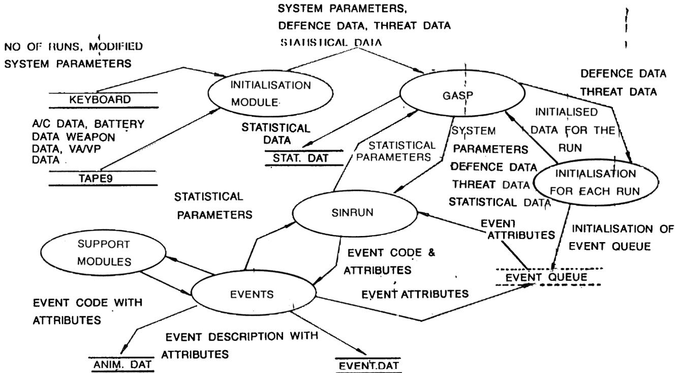
Figure 2. Data flow diagram for Anukalpana 2.0
