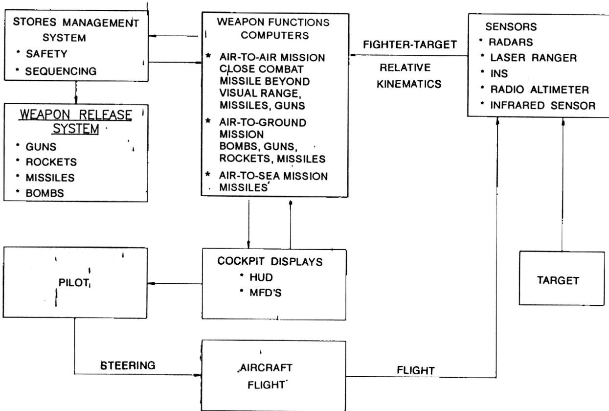
Figure 1. Block diagram of fighter aircraft weapon system
