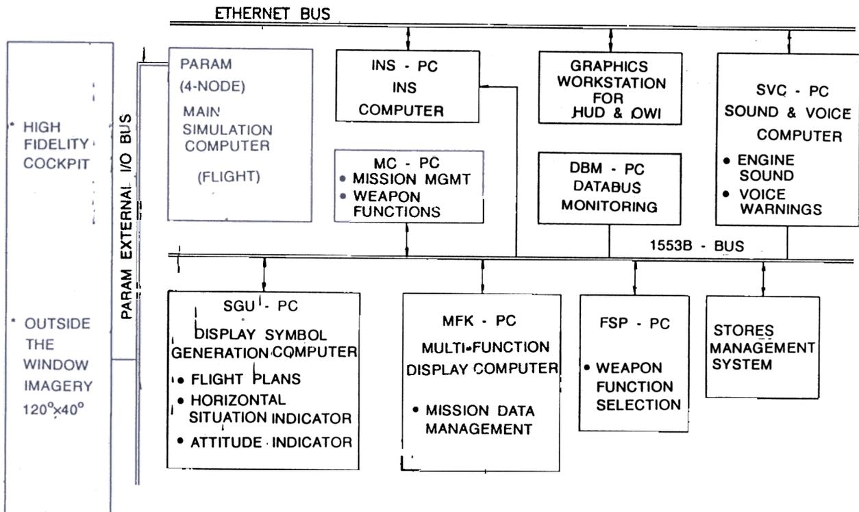
Figure 6. High fidelity cockpit environment facility for weapon system evaluation
