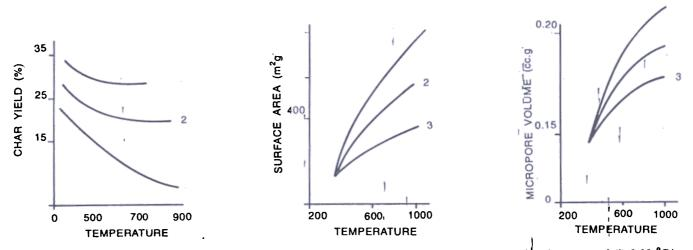
Figure 6. Influence of heating rate on (a) char yield, (b) surface area, (c) micropore yolume at heating rates of (i) 0.03 °C/m (ii) 11 °C/min, and (iii) 70 °C/min (Ref 37).
