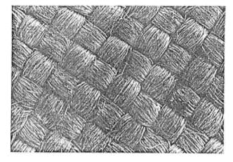
Figure 2. Activated carbon fabric
