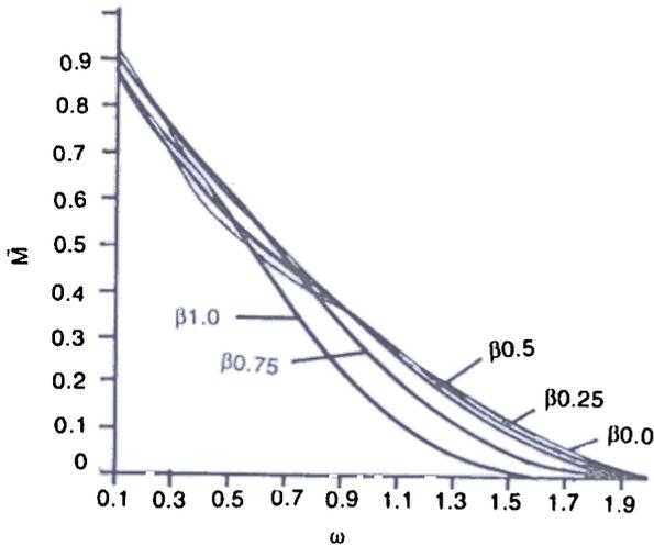
Figure 5. Modulation of triangular targets for  $\alpha = 0.50$
