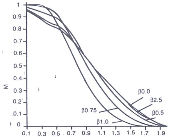
Figure 2. Modulation of rectangular targets for  $\alpha = 0.50$
