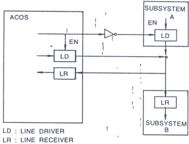
Figure 4. Party line configuration for digital signals
