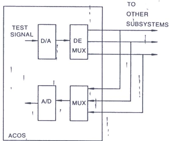
Figure 5. Analog signal loop check
