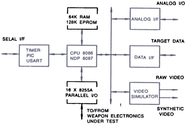
Figure 1. Block diagram of ACOS
