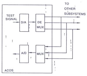
Figure 5. Analog signal loop check
