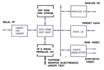
Figure 1. Block diagram of ACOS
