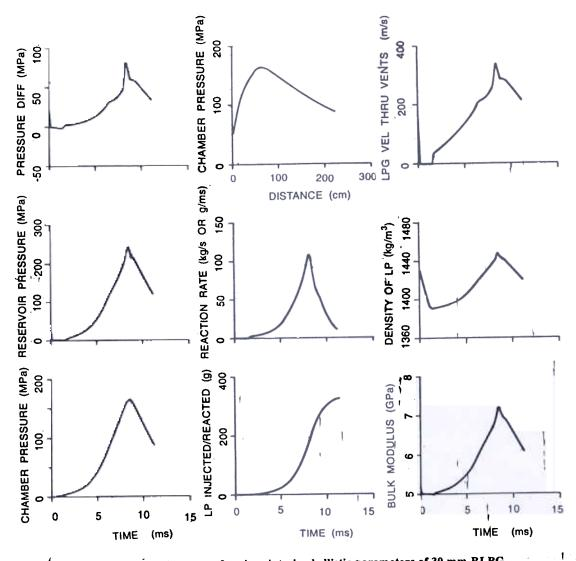
Figure 2. Time development of various int rior ballistic parameters of 30 mm RLPG
