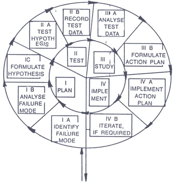
Figure 3. Failure analysis spiral.
