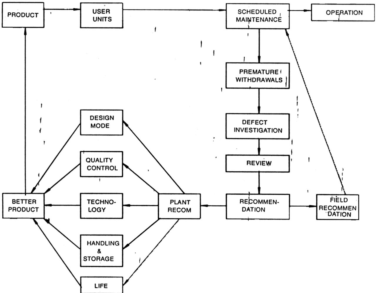
Figure 4. Scheme for defect investigation
