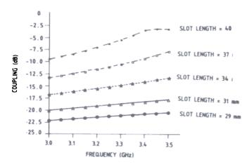
Figure 4. Frequency vs coupling for different slot lengths
