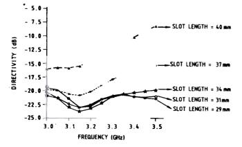
Figure 5. Frequency vs directivity for different slot lengths
