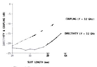
Figure 6. Slot length vs coupling and directivity
