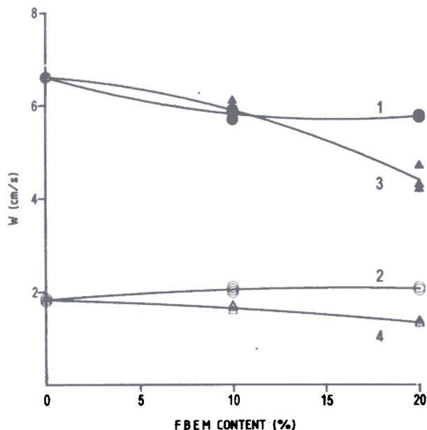
Figure 1. Effect of FBEM content on the burning rate of AP-based composite propellants at 10 MPa. Fast-burning additives: LTNC (1, 2) and LDNP (3, 4). FBEM particle size ( $< 10 \mu\text{m}$ ).
