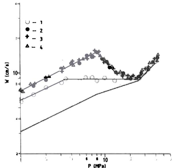
Figure 11. Effect of pressure on the burning rate of a composite propellant containing 15 per cent GP grains. GP particle size:  $< 400 \mu\text{m}$  (1),  $400-800 \mu\text{m}$  (2),  $800-1000 \mu\text{m}$  (3),  $1000-1250 \mu\text{m}$  (4). Solid line without points: base-line propellant.
