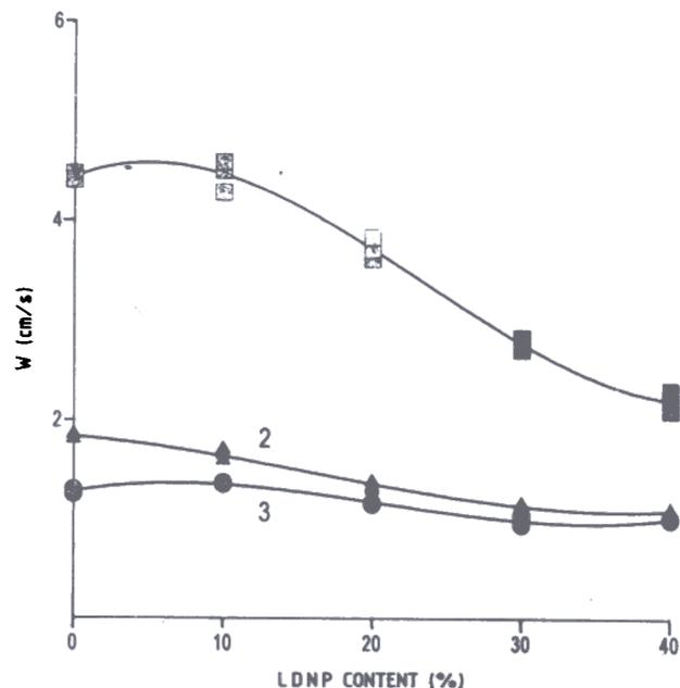
Figure 2. Effect of LDNP content on the burning rate of AP-based composite propellants at 10 MPa. LDNP particle size ( $< 10 \mu\text{m}$ ).
