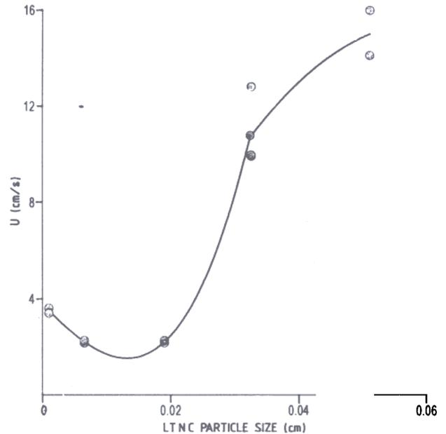
Figure 5. Effect of LTNC particle size on the burning rate of binary mixture with polyester at 10 MPa. Polyester content 20%.
