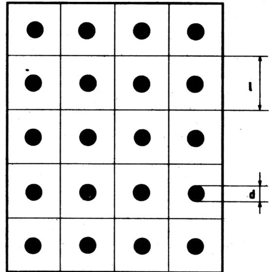
Figure 7. Schematic of distribution of FBEM grains in a propellant composition. ( $l$ ) Size of unit volume, ( $d$ ) - FBEM grain size.
