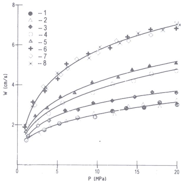
Figure 6. Burning rate vs pressure for a composite propellant containing 15 per cent LTNC grains at different LTNC particle sizes: <math>< 10 \mu\text{m}</math> (2), <math>< 100 \mu\text{m}</math> (3), <math>200\text{--}315 \mu\text{m}</math> (4), <math>315\text{--}400 \mu\text{m}</math> (5), <math>400\text{--}630 \mu\text{m}</math> (6), <math>630\text{--}800 \mu\text{m}</math> (7), <math>800\text{--}1000 \mu\text{m}</math> (8). Base-line propellant (1).
