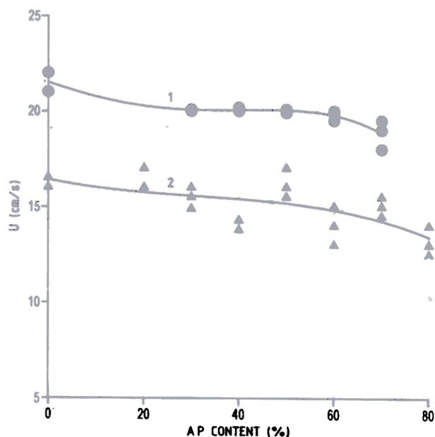
Figure 3. Effect of AP content on the burning rate of binary mixtures with LTNC (1) and LDNP (2) at 10 MPa. AP particle size (160-250  $\mu\text{m}$ ).
