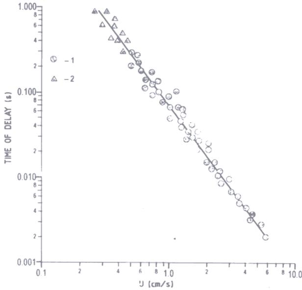
Figure 8. Ignition delay time as a function of the burning rate of AP-based composite propellants (1), and double-base propellants (2).
