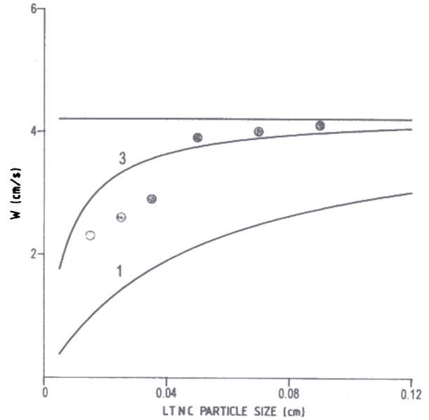
Figure 9. Experimental and calculated burning rates of a composite propellant containing 15 per cent LTNC grains at 4 MPa, as a function of LTNC particle size. Curves calculated from Eqn (8) for  $n = 7 \cdot 10^{-2}$  (1);  $\tau_d = 0$  (2);  $n = 1 \cdot 10^{-2}$  (3).
