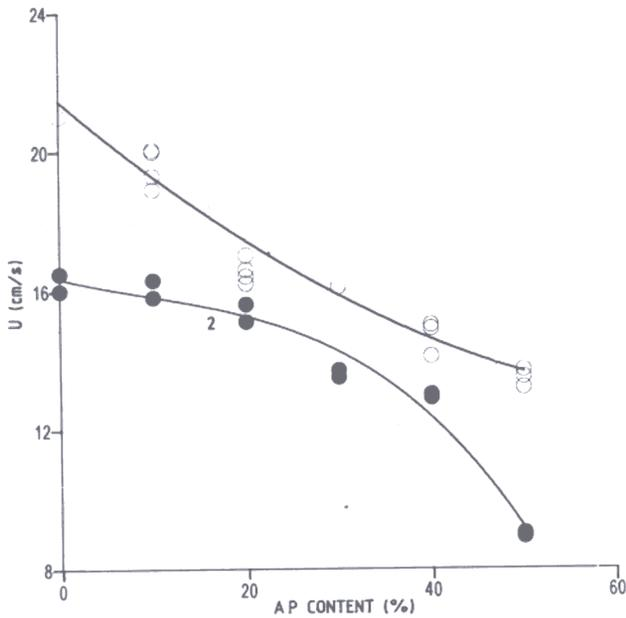
Figure 4. Effect of AP content on the burning rate of binary mixtures with LTNC (1) and LDNP (2) at 10 MPa. AP particle size (approx 1  $\mu\text{m}$ ).
