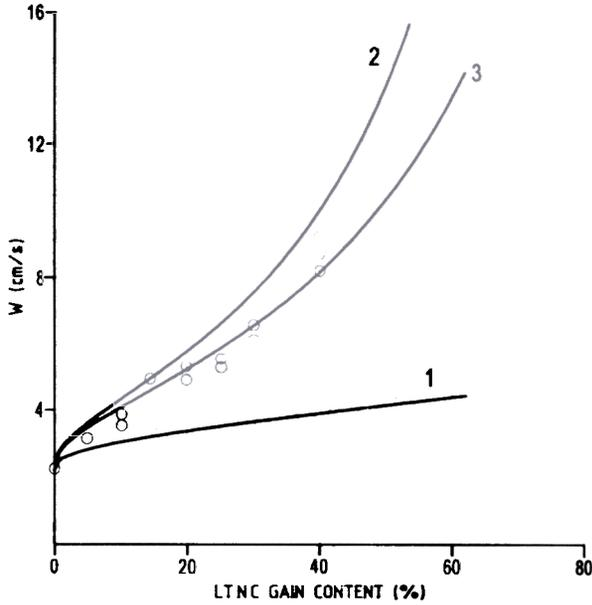
Figure 10. Experimental and calculated burning rates of a composite propellant containing LTNC of 800  $\mu\text{m}$  particle size at 10 MPa, as a function of LTNC content. Curves calculated from Eqn (8) for  $n = 7 \cdot 10^{-2}$  (1);  $\tau_d = 0$  (2);  $n = 1 \cdot 10^{-2}$  (3).
