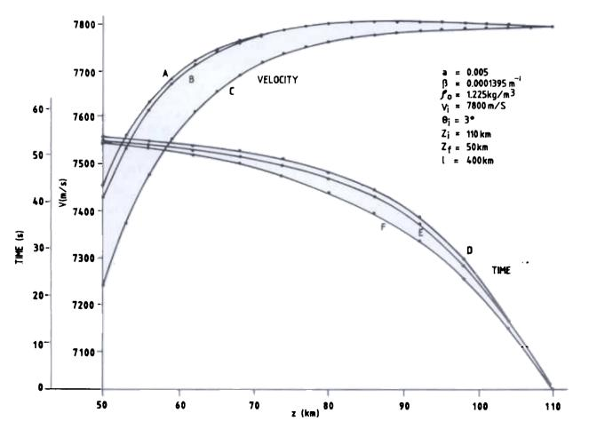
Figure 2. Variation of velocity and time with altitude for minimum time re-entry trajectory (A & D-gravity plus spherical earth; B&E-gravity plus flat earth and C & F-gravity neglected plus flat earth.
