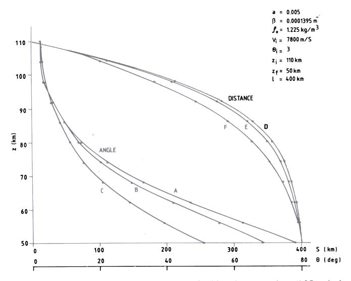
Figure 3. Variation of angle and distance along the horizontal with altitude for minimum time re-entry trajectory (A & D-gravity plus spherical earth; B & E-gravity plus flat earth and C&F-gravity neglected plus flat earth.
