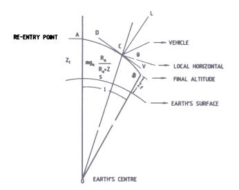
Figure 1. Geometry of the re-entry trajectory
