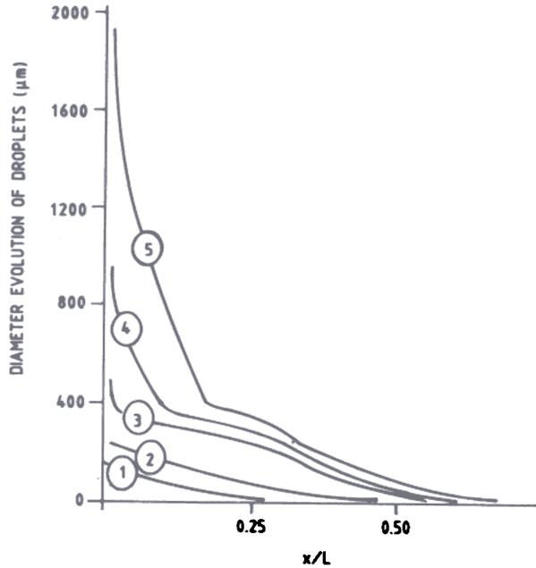
Figure 2. Change in diameter of water droplets over length of channel: (1)  $d = 100 \mu\text{m}$ , (2)  $d = 200 \mu\text{m}$ , (3)  $d = 500 \mu\text{m}$ , (4)  $d = 1000 \mu\text{m}$ , and (5)  $d = 2000 \mu\text{m}$ .
