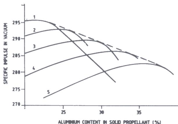
**Figure 1. Vacuum specific impulse vs aluminium content in solid propellant as a function of water content in total mass supply in combustion chamber (water percentage: (1) 0, (2) 5, (3) 10, (4) 15, and (5) 20 %).**
