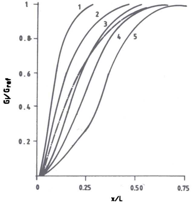
Figure 3. Dimensionless steam supply from particles of fractions 1-5 at different cross-sections of channel: (1)  $d = 100 \mu\text{m}$ , (2)  $d = 200 \mu\text{m}$ , (3)  $d = 500 \mu\text{m}$ , (4)  $d = 1000 \mu\text{m}$ , and (5)  $d = 2000 \mu\text{m}$ . chain line corresponds to total steam supply into the chamber.
