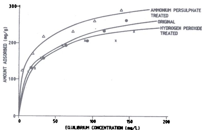
Figure 4. Freundlich adsorption isotherms of trinitrophenol on activated carbon AC-60 (1150 m<sup>2</sup>/g) before and after surface oxidation. Temperature 30 ± 1 °C contact time 24 hr, initial concentration 300 mg/l and carbon dose 0.2-2.0 g/l.
