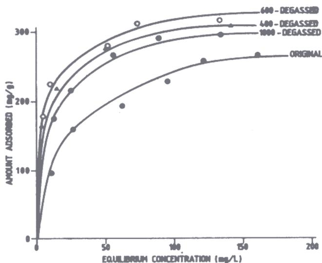
Figure 3. Freundlich adsorption isotherms for trinitrophenol on activated carbon AC-60 (1150 m<sup>2</sup>/g) before and after outgassing at different temperatures. Temperature 30 ± 1 °C, contact time 24 hr, initial concentration 300 mg/l, and carbon dose 0.2-2.0 g/l.
