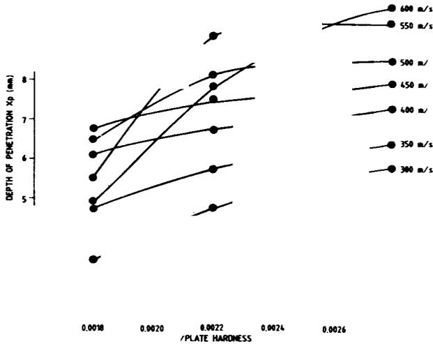
Figure 9. Variation of depth of penetration with 1/ plate hardness.
