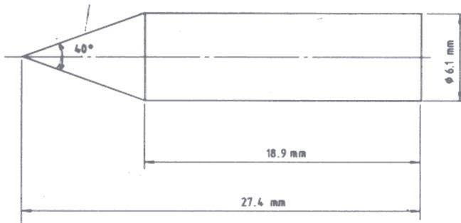
Figure 1. Projectile detail
