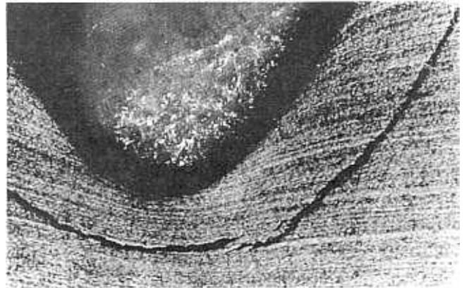
Figure 6. Sectioned surface of a crater on 450 Hv plate showing deep crack around the periphery of the impacted hole by a steel projectile at zero obliquity.
