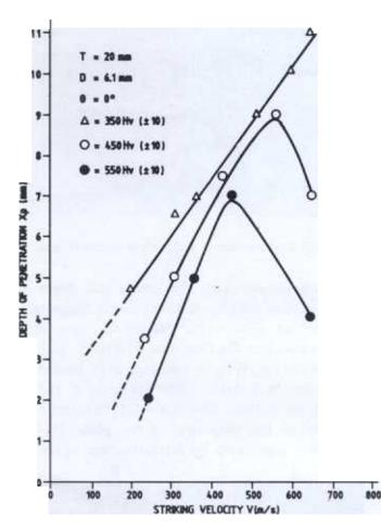
Figure 7. Variation of depth of penetration with striking velocity of 20 mm thick tempered steel armour plates (350, 450 and 550 Hv) at zero obliquity.
