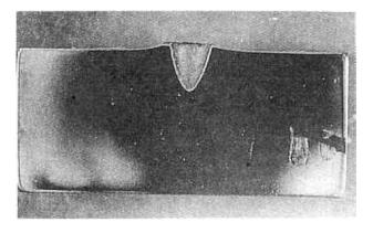
Figure 5. Lip formation on entry side of the 350 Hv plate
