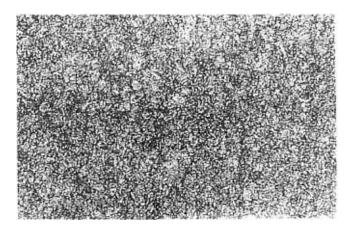
Figure 2. Microstructure of tempered 20 mm thick steel plate at 200 X (350 Hv).
