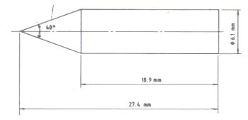
Figure 1. Projectile detail
