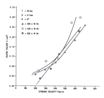
Figure 8. Variation of crater volume with striking velocity of 20 mm thick steel armour plates (350, 450 and 550 Hv) at zero obliquity.
