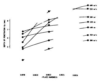
Figure 9. Variation of depth of penetration with 1/ plate hardness.
