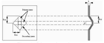
Figure 1. Primary and secondary yarns.
