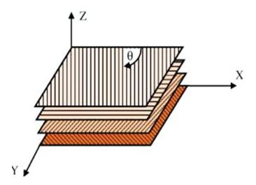
Figure 2. Principal directions of the laminate.
