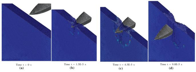
Figure 4. Damage propagation in (0/90) lay-up 19 layer glass/epoxy plate.
