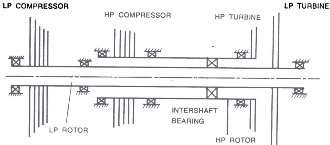
Figure 1. Schematic of a two-spool aeroengine rotor
