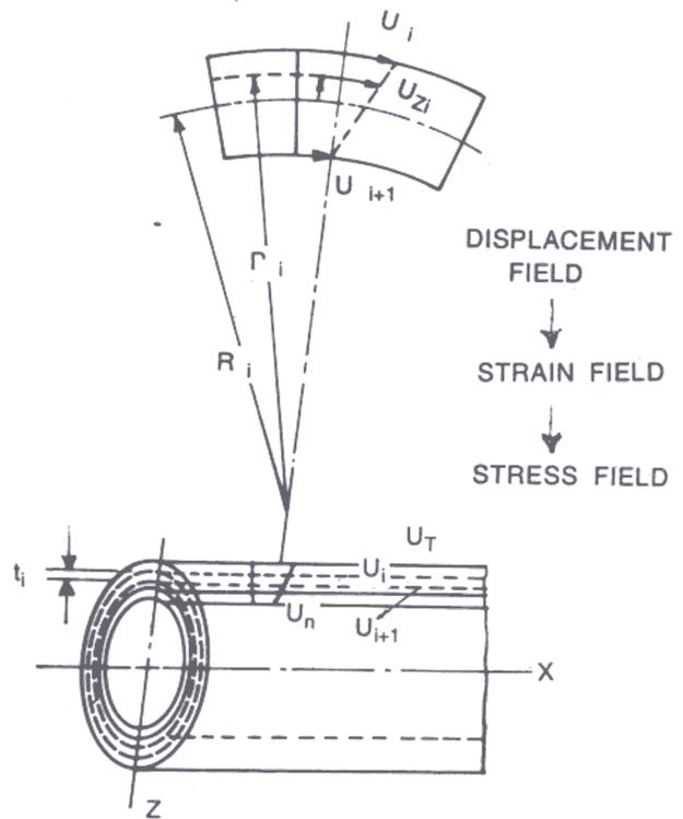
Figure 5. Layerwise approach for stress analysis of shaft
