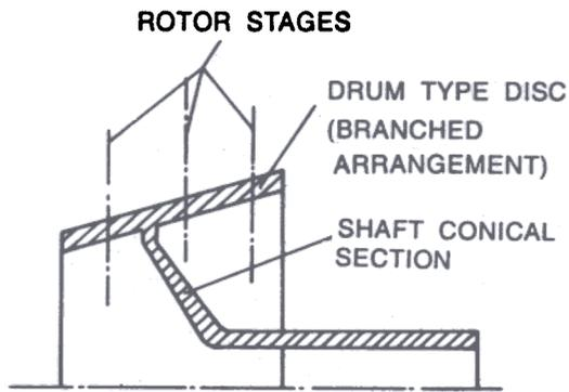
Figure 3. Schematic of branched arrangement and shaft conical section.
