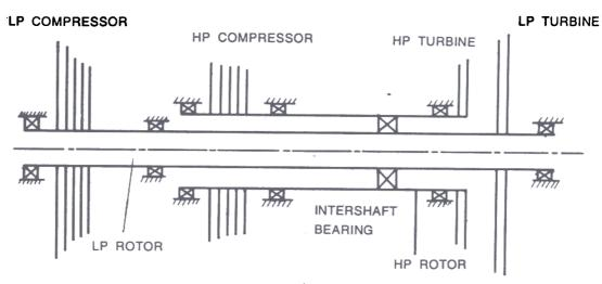
Figure 1. Schematic of a two-spool aeroengine rotor
