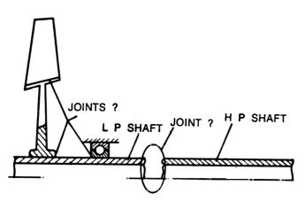
Figure 4. Difficulties in joining of components and mounting of rotors.
