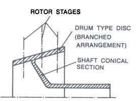
Figure 3. Schematic of branched arrangement and shaft conical section.
