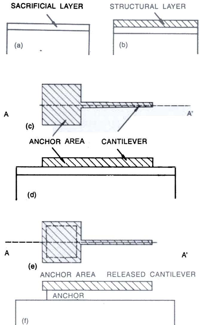
Figure 5. Schematic demonstration of surface micromachining: (a) cross-sectional view after the sacrificial layer is deposited, (b) cross-sectional view after the structural layer is deposited, (c) top plan view after patterning of the structural layer, (d) cross-section AA' of (c); (e) top plan view after release, and (f) cross-section AA' of (e).
