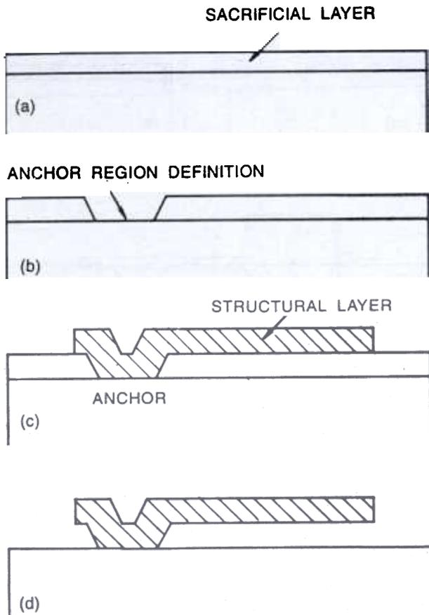
Figure 6. Cross-sectional schematics demonstrating the addition of an anchor definition step: (a) after the sacrificial layer is deposited, (b) after the anchor region is defined, (c) after patterning the structural layer, and (d) after release.
