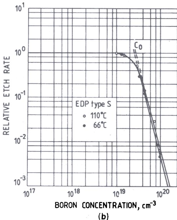
Figure 3. Relative *Si* etch as a function of *B* dopant concentration for (a) various *KOH* solutions, and (b) EDP.
