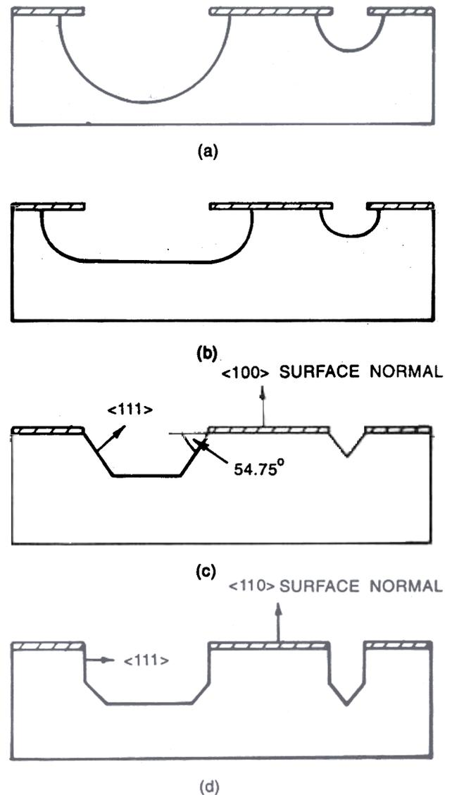
Figure 1. Summary of wet chemically-etched hole geometries commonly used in micromechanical devices: (a) isotropic etching without agitation, (b) isotropic etching with agitation, (c) anisotropic etching on (100) surfaces, (d) anisotropic etching on (110) surfaces.
