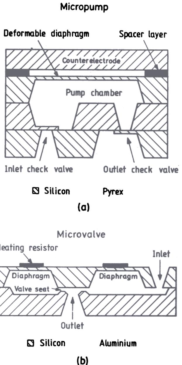
Figure 4. Cross-section of (a) an electrostatic diaphragm micropump, and (b) a bimetallic diaphragm microvalve fabricated by *Si* fusion bonding of four and two *Si* wafers, respectively.
