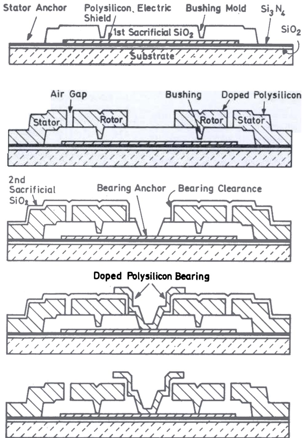
Figure 7. Schematic drawing demonstrating surface micromachining of a micrometer: (a) after the bushing mold and stator anchor are patterned, (b) after the rotor and stator are patterned, (c) after the bearing anchor is patterned, (d) after the bearing is patterned, and (e) completed device.
