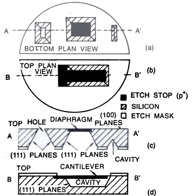
Figure 2. Schematic drawing of bulk micromachining: (a) bottom plan view of anisotropically etched wafer showing the fabrication of cavities, diaphragms and holes, (b) top plan view of anisotropically etched wafer showing the fabrication of a cantilever beam using etch-stop layers. (c) cross-section, AA' showing the hole, diaphragm and cavity of (a), (d) cross section, BB' showing the cantilever beam of (b).
