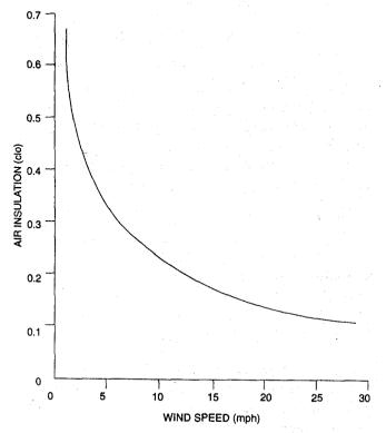
Figure 3. Effect of wind speed on air insulation
