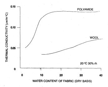
Figure 1. Effect of moisture content on thermal conductivity
