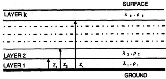
Figure 7. Layered snowpack [ $z_i, \rho_i, \lambda_i$  are the height, density and the conductivity, respectively of layer  $i$ ].
