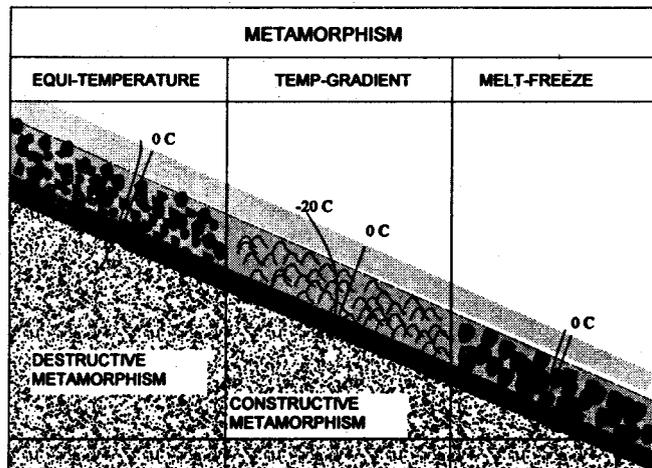
Figure 4. Process of metamorphism occurring within the snowcover.
