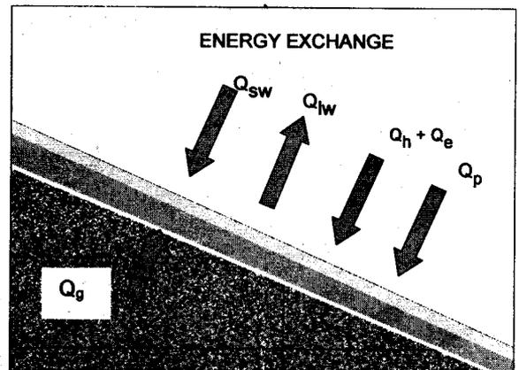
Figure 2. Energy exchange between snowcover and surroundings.
