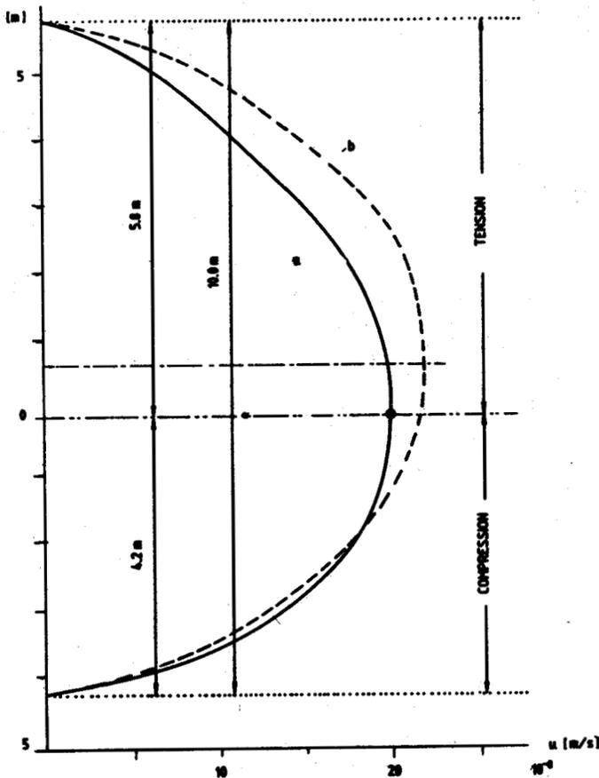
Figure 5. Creep velocity distribution of the overburden snow layer within the super-weak zone (a-nonlinear, b-linear)
