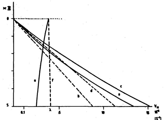
Figure 1. Deformation rates in a uniform horizontal snowcover under compression. Uniaxial state of deformation: a-nonlinear, b-linear; uniaxial state of stress: c-nonlinear, d-linear;  $\lambda$  values: e-nonlinear, f-linear.
