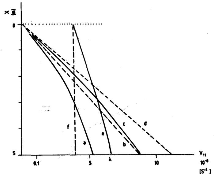
Figure 2. Deformation rates in a uniform horizontal snowcover under tension (imaginary). Uniaxial state of deformation: a-nonlinear, b-linear; uniaxial state of stress: c-nonlinear, d-linear;  $\lambda$  values: e-nonlinear, f-linear.
