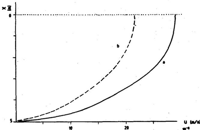
Figure 3. Creep velocities in a uniform horizontal snowcover under compression (settlement).
