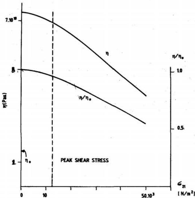
Figure 6. Stress-dependent viscosity according to Eqn (34).  $\eta_0$ : linear viscosity (small shear stresses. Peak shear stress according to Eqn (32).
