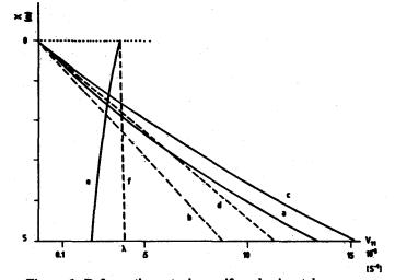
Figure 1. Deformation rates in a uniform horizontal snowcover under compression. Uniaxial state of deformation: *a*-nonlinear, *b*-linear; uniaxial state of stress: *c*nonlinear, *d*-linear; λ values: *e*-nonlinear, *f*-linear.
