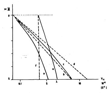
Figure 2. Deformation rates in a uniform horizontal snowcover under tension (imaginary). Uniaxial state of deformation: a-nonlinear, b-linear; uniaxial state of stress: c-nonlinear, d-linear; λ values: e-nonlinear, f-linear.
