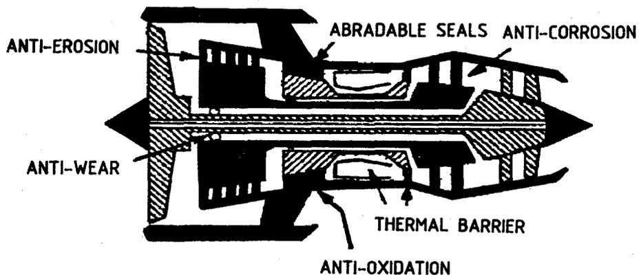
Figure 1. Typical areas of coating application
