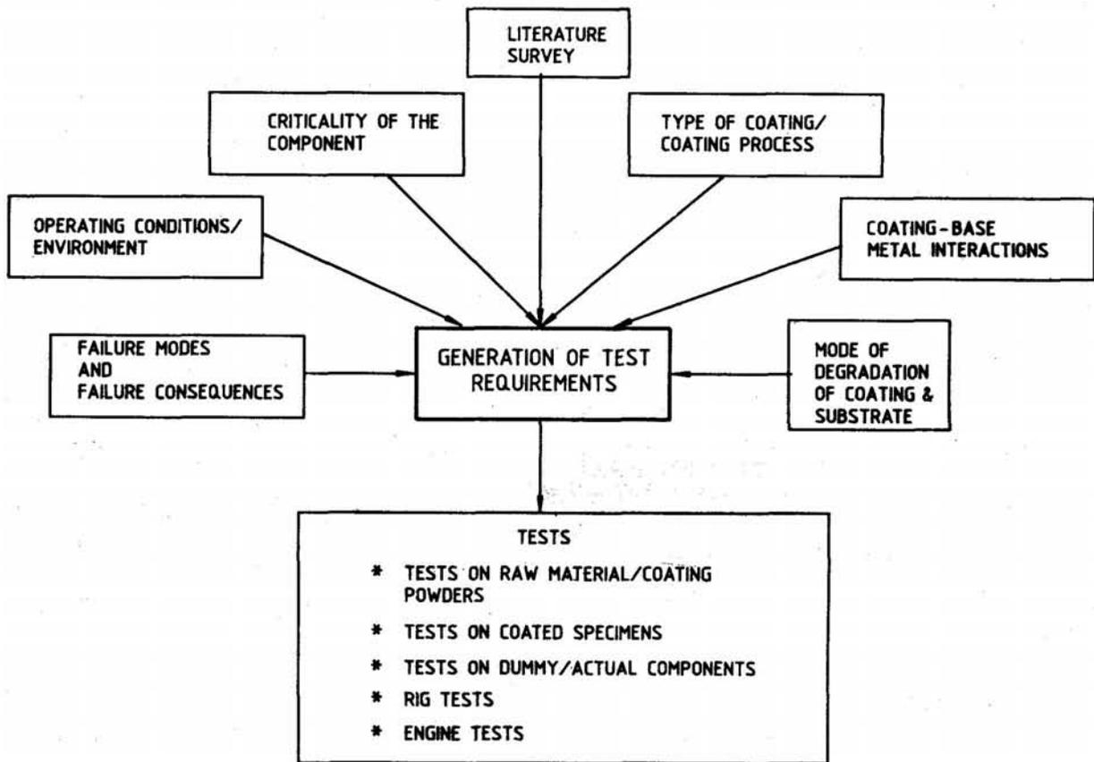
Figure 4. Evolution of test requirements
