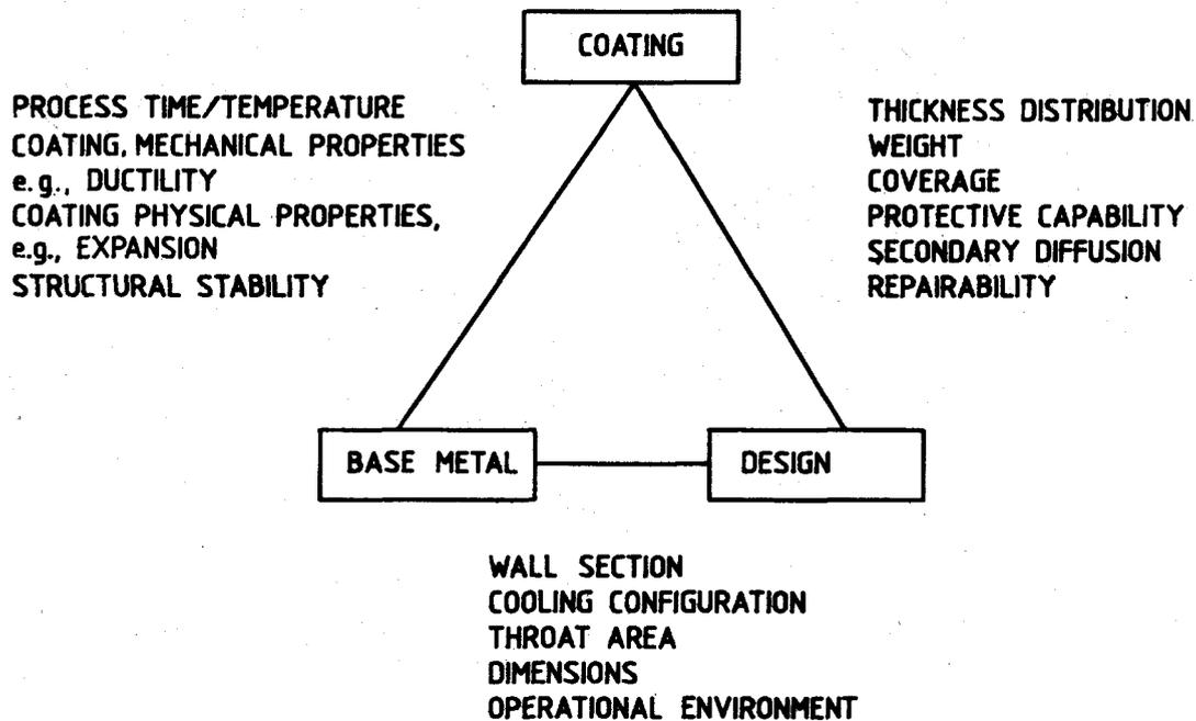
Figure 2. Interaction of coating, base material and design considerations
