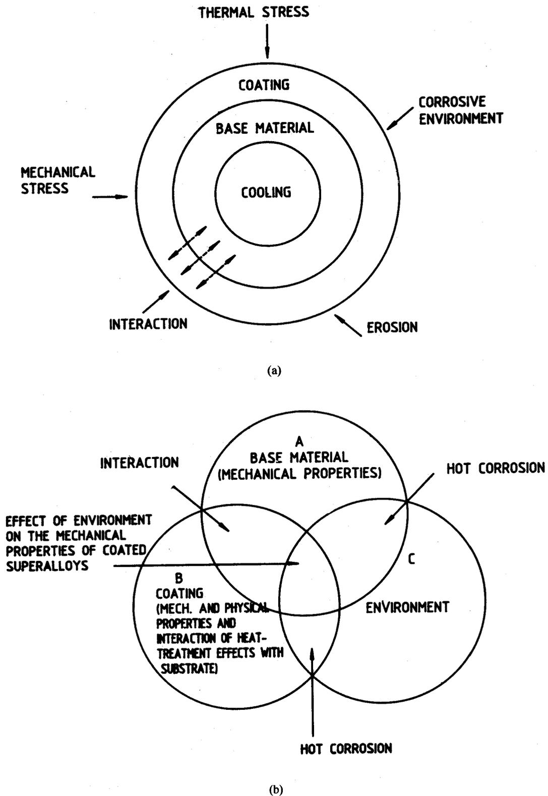
Figure 3. Factors determining effectiveness of coating: (a) substrate and coating, and (b) substrate, coating, and environment
