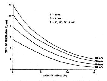
Figure 4. Variation of depth of penetration with the obliquity
