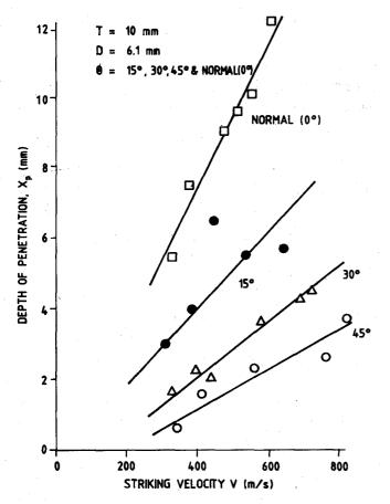
Figure 1. Variation of depth of penetration with velocity at different angles of attack (obliquity).
