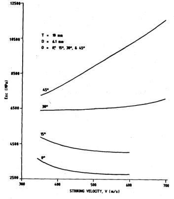
Figure 3. Variation of plate resistance with projectile velocity at different angles of attack.
