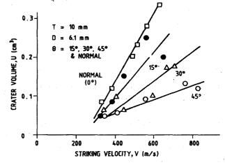
Figure 2. Variation of crater volume with projectile velocity at different angles of attack (obliquity).
