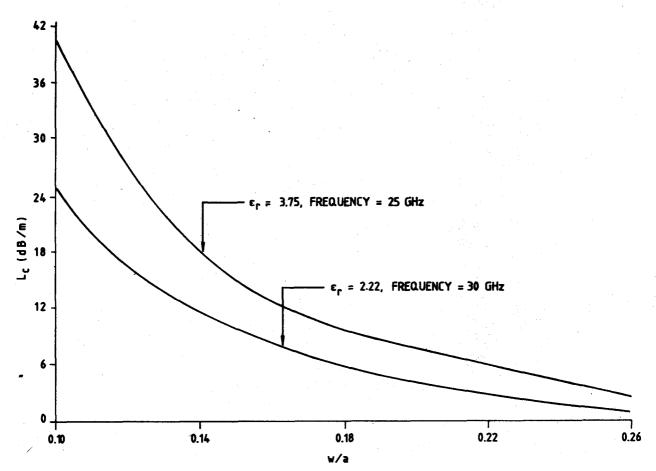
Figure 5. Conduction loss vs slot width
