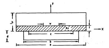
Figure 1. Cross-section of pedestal-supported bilateral finline
