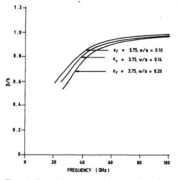
Figure 4. Propagation constant vs frequency for various values of w/a.
