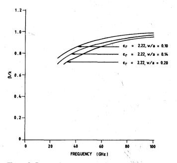
Figure 3. Propagation constant vs frequency for various values of w/a.
