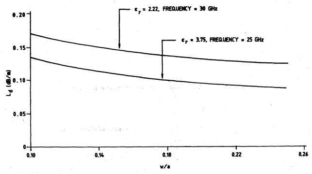
Figure 6. Dielectric loss vs slot width
