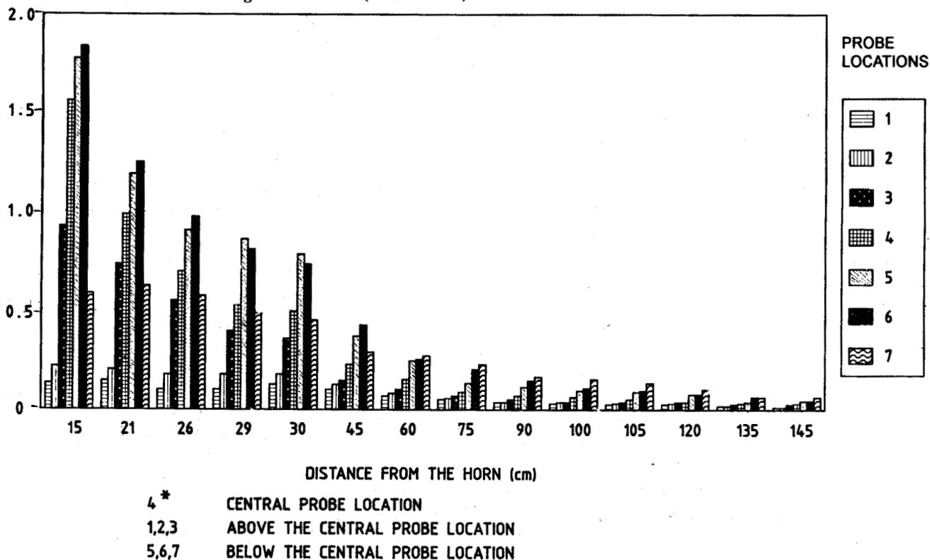
Figure 3(b). Mean values of X-axis/vertical axis readings ( $mW/cm^2$ ) at various distances from the helmet-mounted microwave radiating horn antenna (helmet No. 2).
