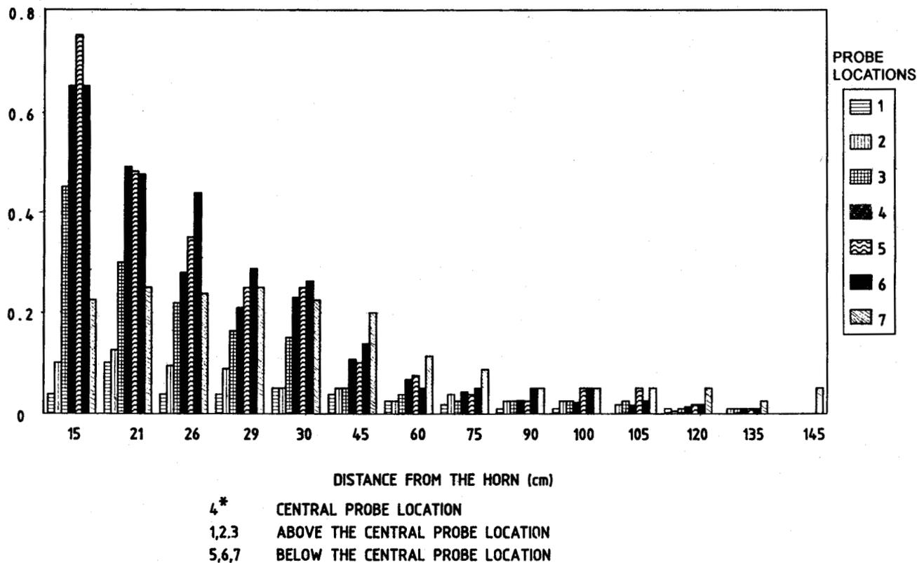
Figure 3(a). Mean values of X-axis/vertical axis readings ( $mW/cm^2$ ) at various distances from the helmet-mounted microwave radiating horn antenna (helmet No. 1).
