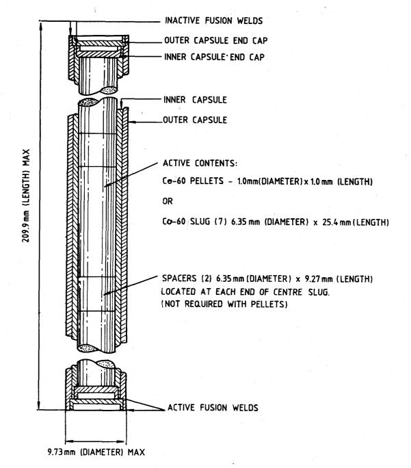
Figure 1. Geometry of the needle sources inside the gamma chamber
