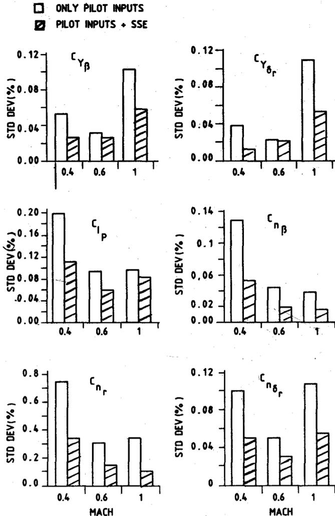
Figure 5. Standard deviation of estimated parameters with and without SSE.
