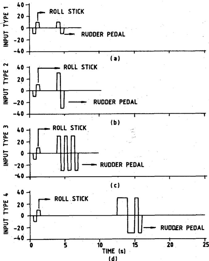
Figure 1. Types of pilot inputs, (a) similar doublet inputs to roll stick and rudder, (b) doublet input with increased amplitude to rudder, (c) repeated doublets input with increased amplitude to rudder, (d) and 3 2 1 1 input with increased amplitude to rudder.
