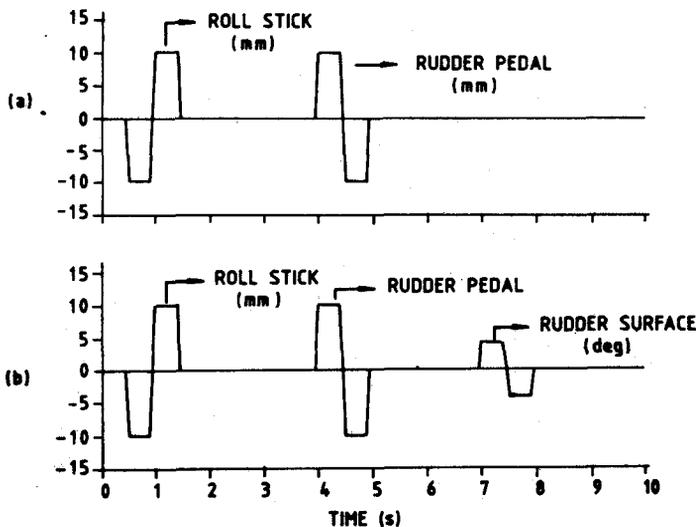
Figure 4. Pilot inputs with SSE, (a) only pilot inputs, and (b) pilot inputs + SSE.
