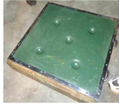
Figure 1. Backing material fixture filled with polymeric clay.
