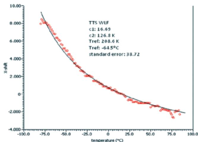
Figure 5. Time-temperature superposition WLF for type-I propellant.
