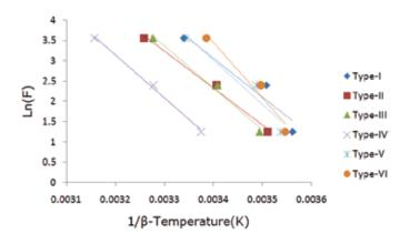
Figure 3. Arrhenius plot of α-transition for each propellant.
