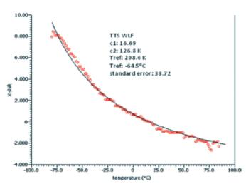
Figure 5. Time-temperature superposition WLF for type-I propellant.
