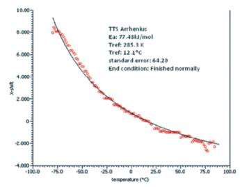
Figure 6. Time-Temperature Superposition (TTS) Arrhenius for type-I Propellant.
