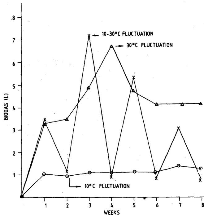
Figure 1. Effect of temperature on biogas production
