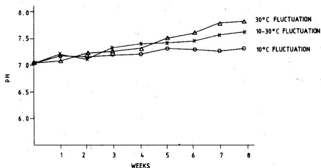
Figure 2. Effect of temperature on pH profile
